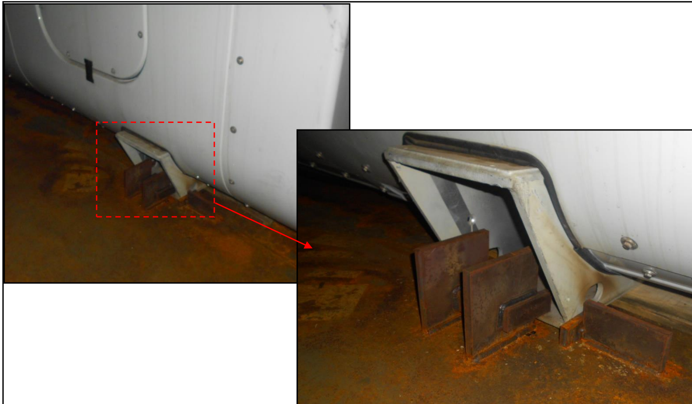
Figure 9: Cargo stoppers applied to wind turbine nacelle unit
