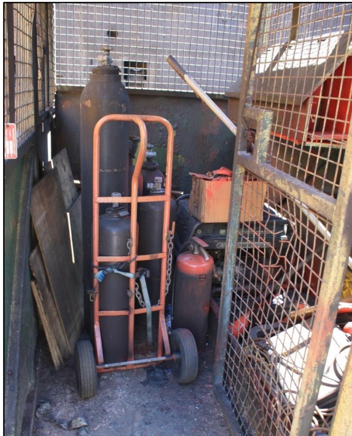
Figure 12: Equipment cage and gas bottles that were in number 2 cargo hold during the fire
