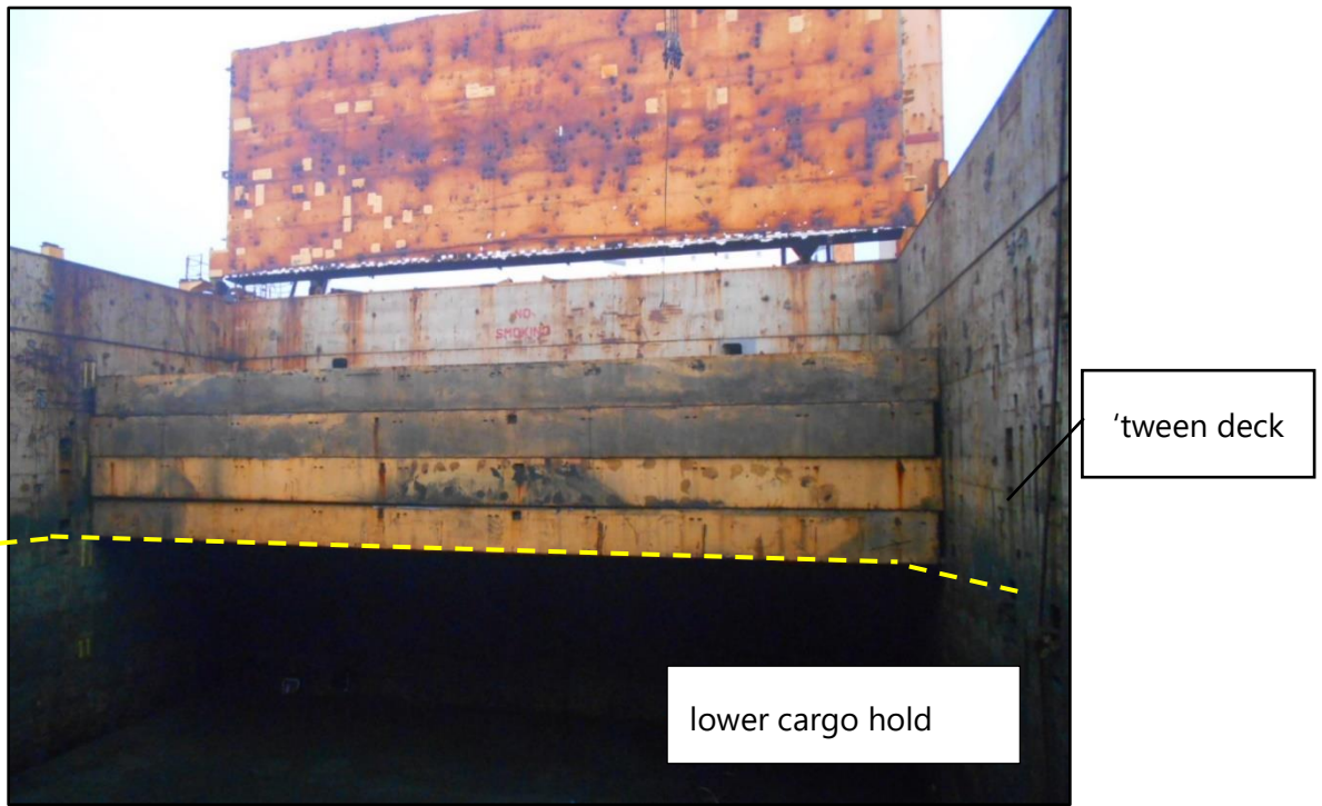
Figure 4: Pontoons stacked and ready to divide a cargo hold into a 'tween deck and lower hold (Credit: Pacific International Lines)
