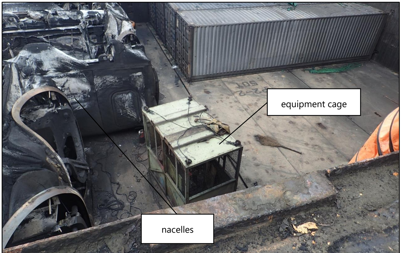
Figure 10: Number 2 'tween deck cargo damage looking from starboard 23 to port 24
