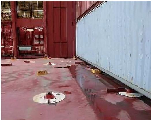
Photograph 22 Pontoon covers on container vessel properly marked/indicated
