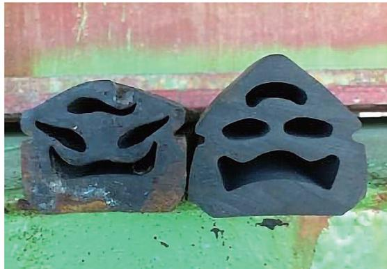
Photograph 9 Overcompressed CAT seal
