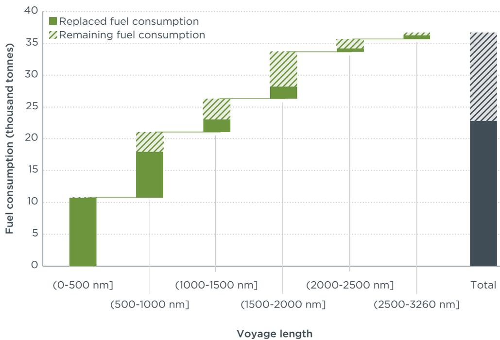
**Figure 4.** Cumulative fuel consumption, replaceable and not replaceable by LH<sub>2</sub>, by voyage length for fishing vessels in the Aleutian Islands.
