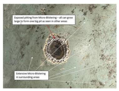
Ship operators should investigate any tanks that meet the above criteria and have had a prolonged period of non-use during a period of reduced operational status. It is recommended that class-related tank inspection due dates are advanced in their survey schedule. Associated piping systems should also be monitored as far as practicable for possible diminution or leakage.
