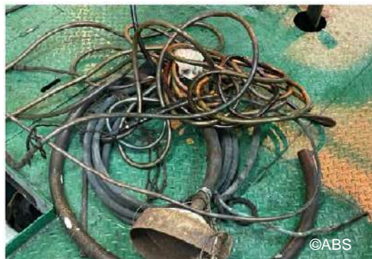
Suspect hoses for unauthorized transfer of oil
