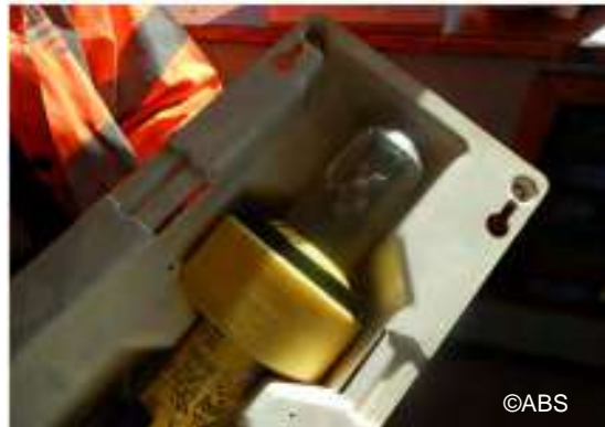
SART located in Bridge with shell cracked, and damaged and not watertight
