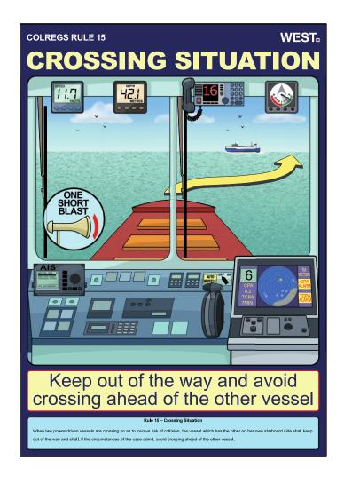
Figure 7: COLREGS Rule 15 Crossing Situation (Credit: West of England Protection and Indemnity provider)
