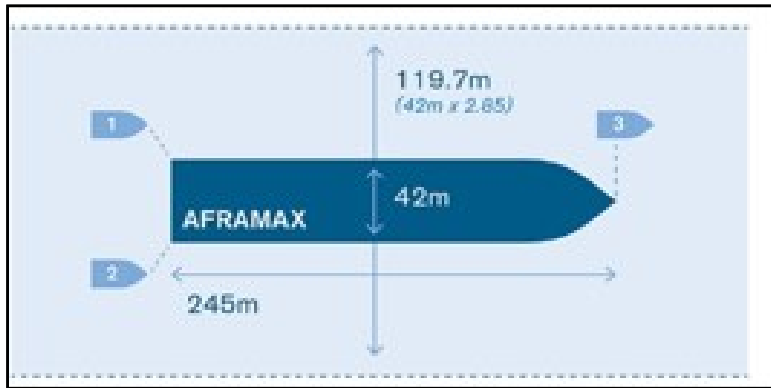
Image: Example of the horizontal channel boundary for a 42m moulded breadth vessel.
