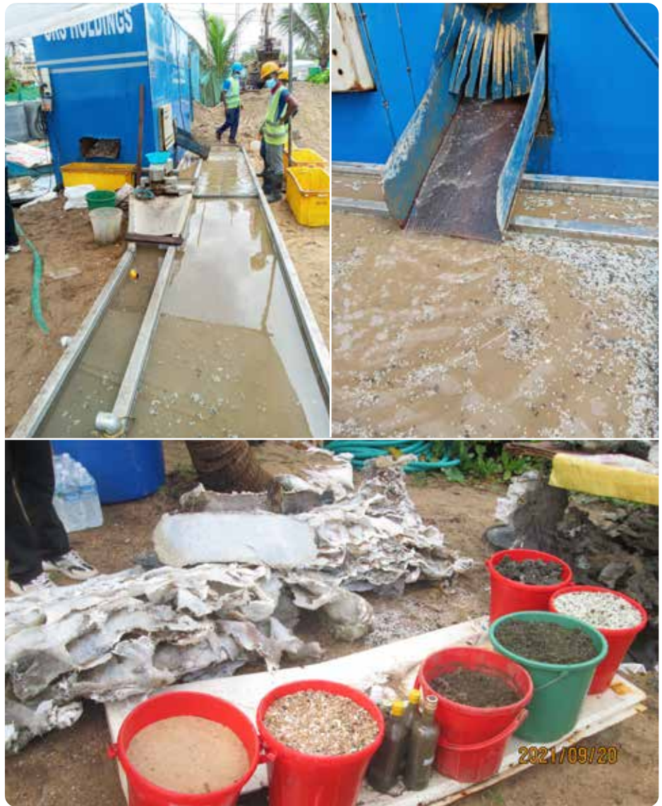
The blue machine operated by Mr. Chinthaka Waragoda that separates out six distinct types of contaminants. The last picture also shows the final cleaned-up sand, and sand with seashells that will go back to the beach. Photos: Panduka Rubesinghe, Harshani Abayawardhana
