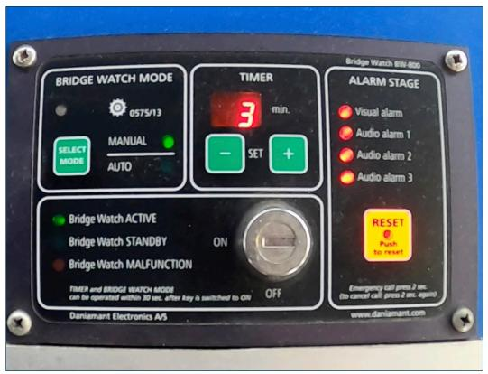
Figure 10: BNWAS during DMAIB test procedure. Source: DMAIB
