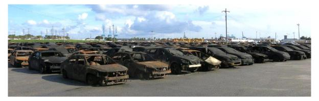
**Figure 7.** Thermally damaged vehicles after removal from the *Höegh Xiamen*, Blount Island, Jacksonville, Florida, July 23, 2020.
