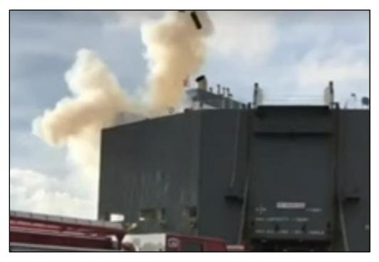
**Figure 5.** Explosion of deck 9 ventilation exhaust housing. Note debris in air at top center of image. (Source: WJXT)
