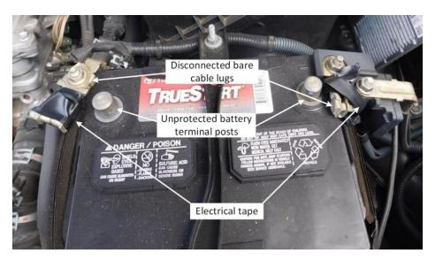
**Figure 14.** Battery in forklift vehicle removed from deck 5. The disconnected battery cable lugs were located near terminal posts, and the battery terminal posts were unprotected. (Source: Coast Guard)
