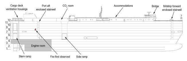
**Figure 3.** Höegh Xiamen inboard profile. (Background source: Höegh Technical Management)
