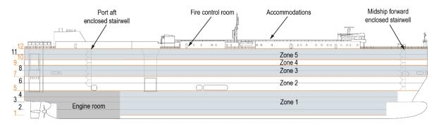
**Figure 8.** Höegh Xiamen fire zones. The vessel's gastight decks, which separate fire zones, are highlighted orange. (Background source: Höegh)
