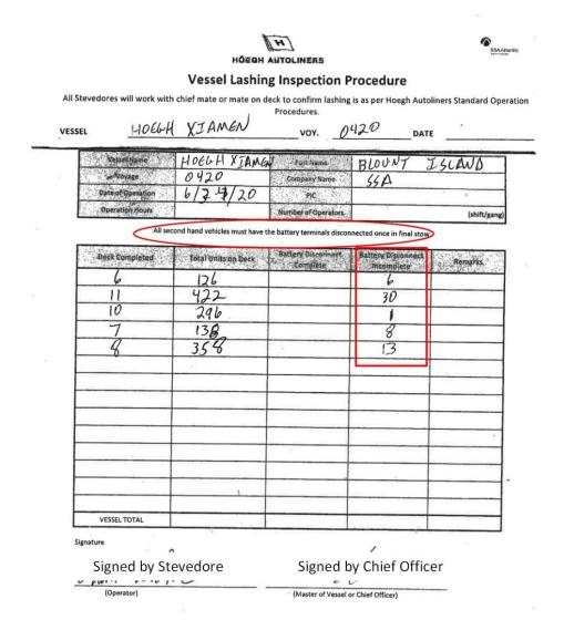
**Figure 13.** Completed "Vehicle Lashing Inspection Procedure." The document states "all second hand [sic] vehicles must have the battery terminals disconnected once in final stow" (red oval) and lists the number of batteries on each cargo deck for which the disconnection was "incomplete" (red rectangle) for the accident loading.
