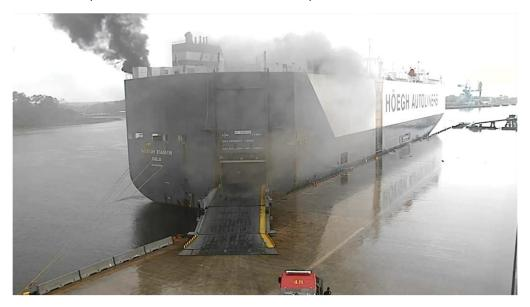
Figure 4. Smoke coming from aft cargo deck ventilation housing exhausts about 1603.
