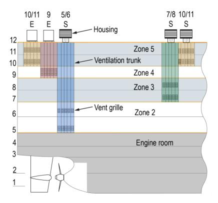
**Figure 10.** Arrangement of portside aft cargo ventilation trunks on deck 12. Each exhaust is marked with an "E," and each supply is marked with an "S." This only represents a portion of the exhaust and supply ventilation trunks.
