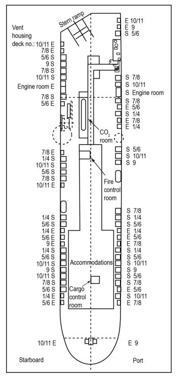
**Figure 9.** Diagram of deck 12 showing ventilation housings. Each exhaust is marked with an "E," and each supply is marked with an "S."
