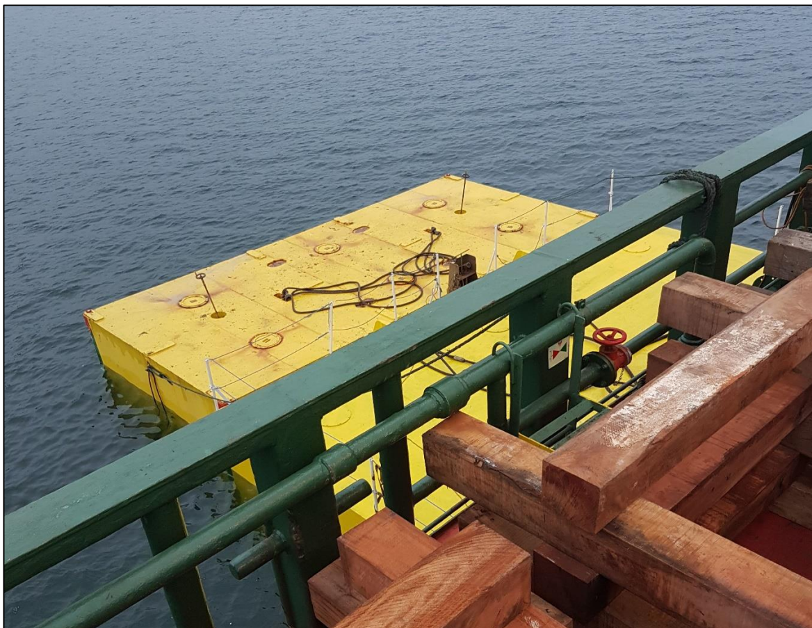
Figure 7: Stabilising pontoon in the water
