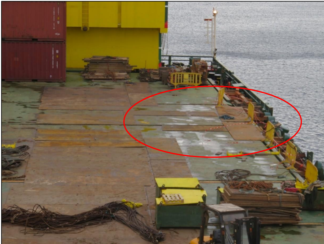
Figure 19: Position of the steel plates on deck after the accident (view to aft)
