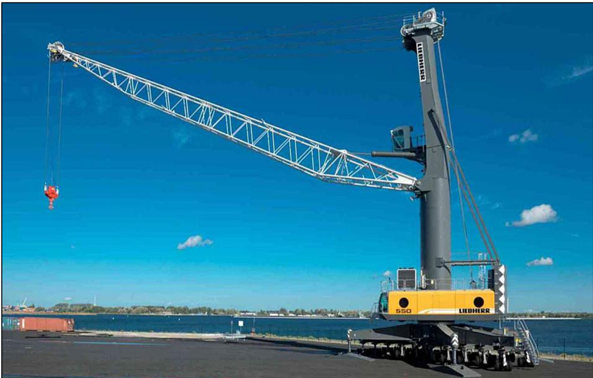
Figure 4: Liebherr LHM 550 ready for use On the models loaded, the hoist cables and hooks were absent and the supporting pads at each corner were implemented twice.
