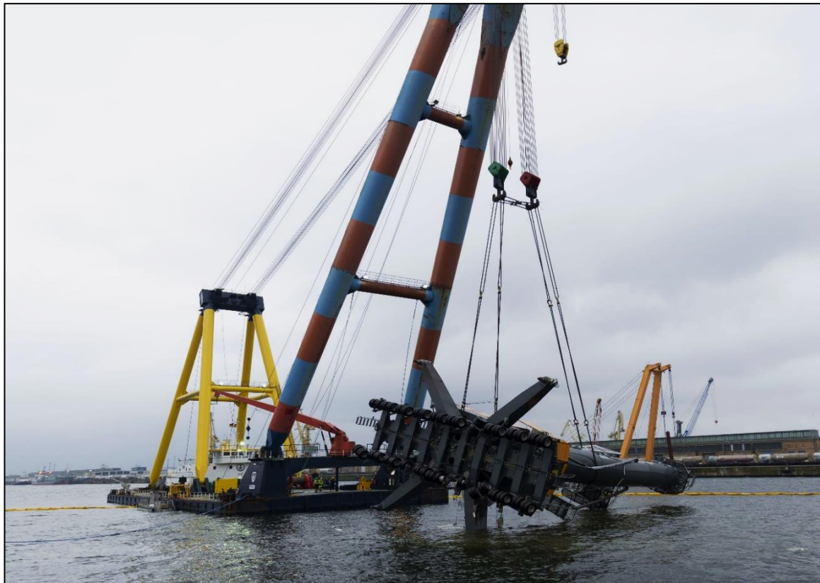
Figure 15: The HEBO LIFT salvaging one of the LHM 550s
