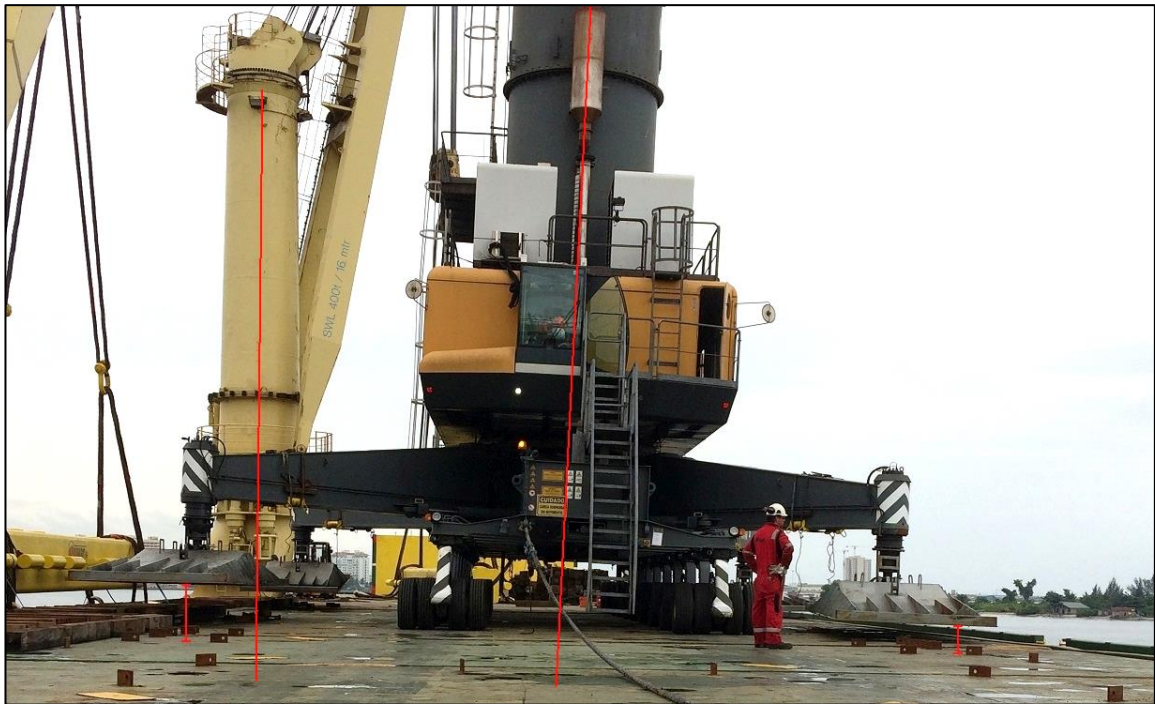
Figure 22: Loading of LHM 550 cranes on the following voyage (view of deck area) The tower of the ship's cargo-handling gear and that of the Liebherr crane are not parallel; the equally extended support cylinders have different distances from the deck
