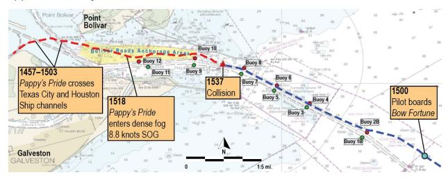
Figure 3. Pappy's Pride outbound track from Galveston (red) and Bow Fortune inbound track (blue) just before the collision. (Source: trackline data Coast Guard, background NOAA.)
