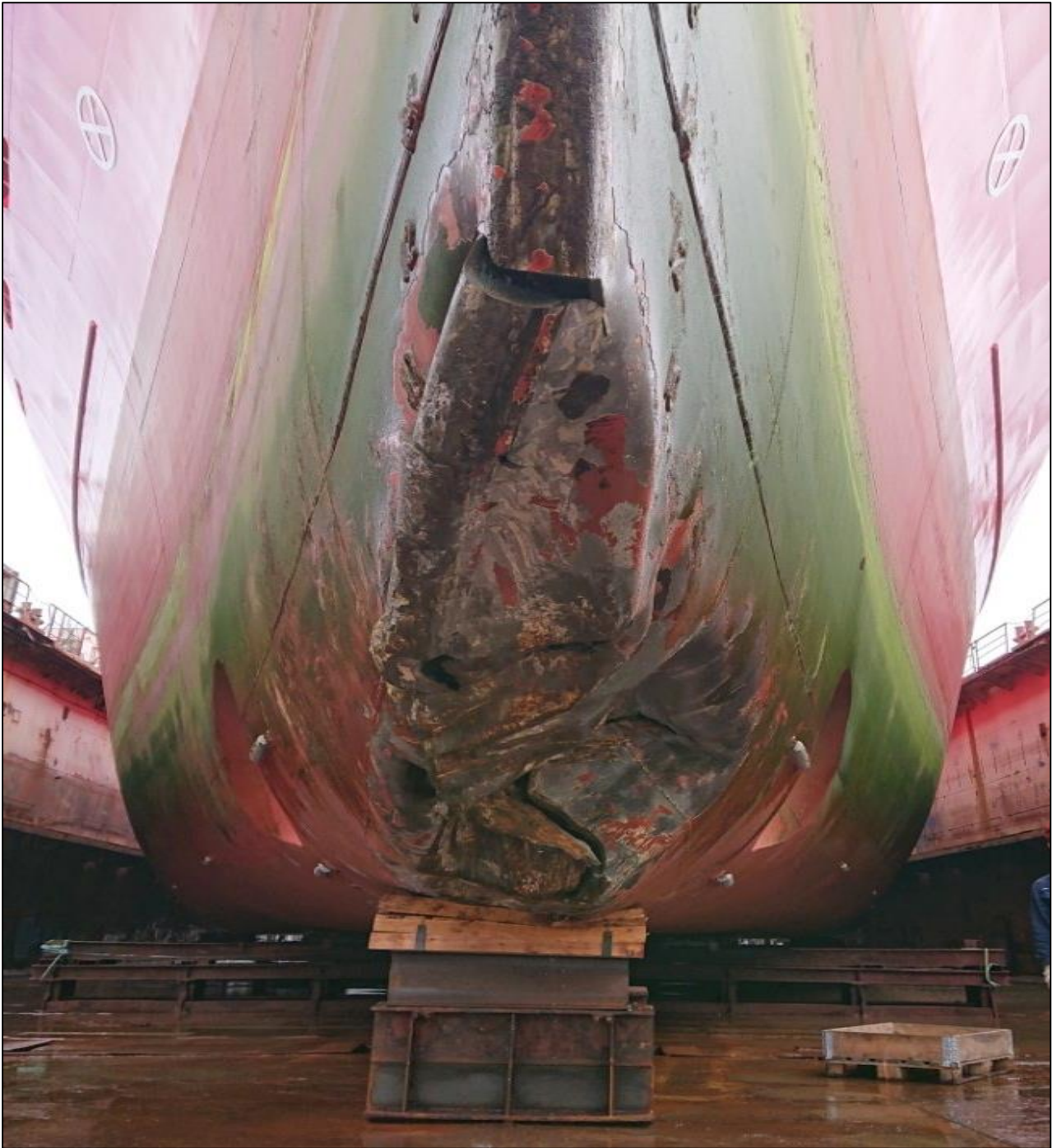
Figure 4: Structural damage to the vessel's stem and hull
