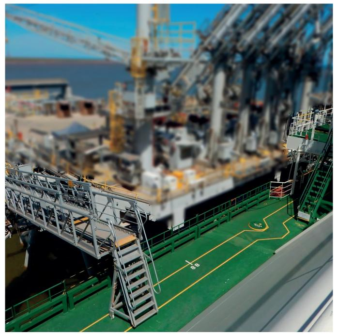
Figure 10: Transverse exit deck ladder
