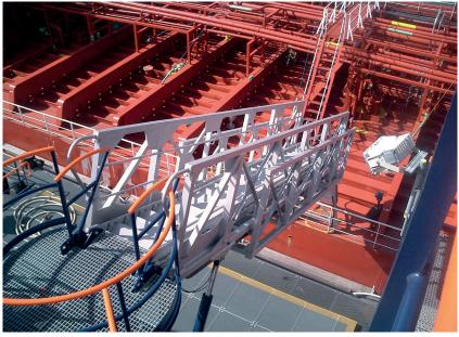
Figure 6: Insufficient landing space on ship deck
