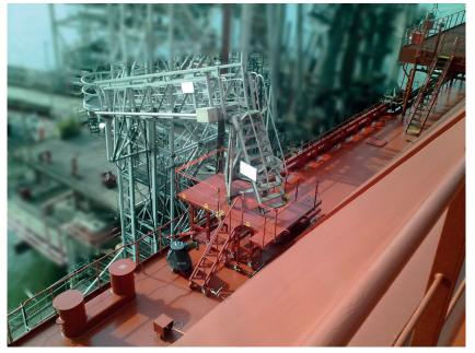
Figure 7: Temporary portable platform over obstructive deck fittings
