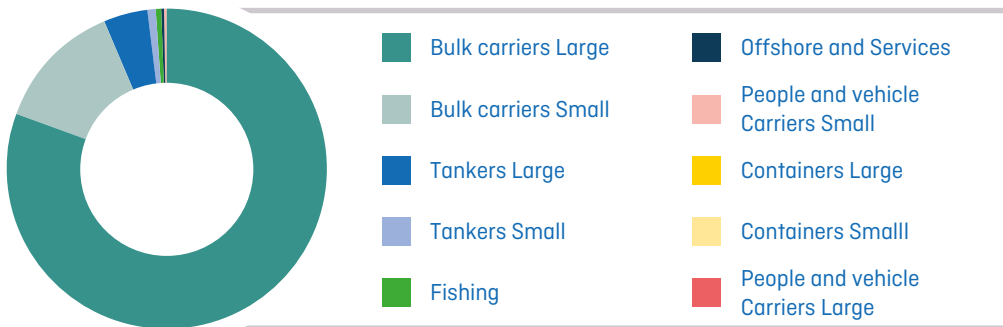
Exhibit 11 - Fuel energy requirement of vessels departing Saldanha Bay by vessel category (vessel category definitions can be found in Appendix C)
