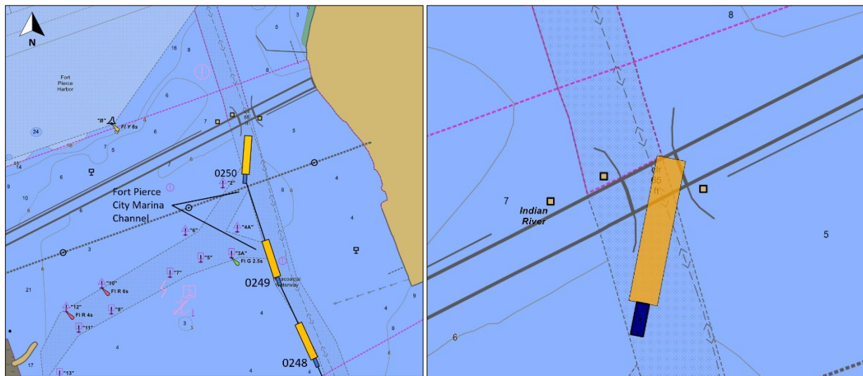
Left: AIS trackline of the Old Glory and Cole outside of and alongside the western boundary of the ICW. (Source: Portvision) Right: The approximate position of the tow after striking the protective fendering system under the Peter P. Cobb Memorial Bridge. (Source: National Oceanic and Atmospheric Administration [NOAA] electronic navigation chart USFL88M)
