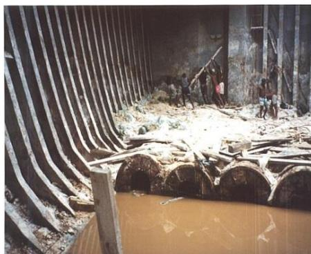
Figure 1: Cargo damage due to water ingress
