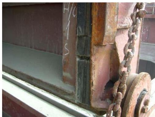
Figure 6: Section replacement of rubber seal
