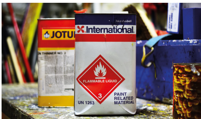
Figure 5: Fuel source stored above flashpoint temperature
