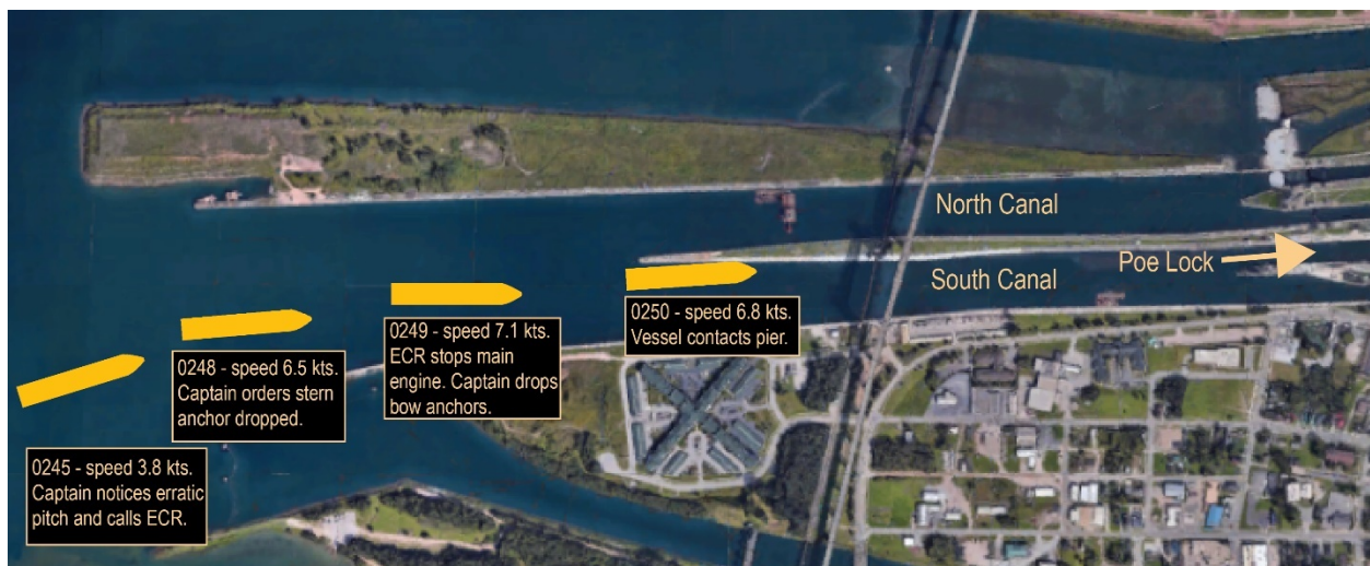
Five-minute accident sequence showing the Atlantic Huron's approach to the west center pier. (Background source: Google Earth)
