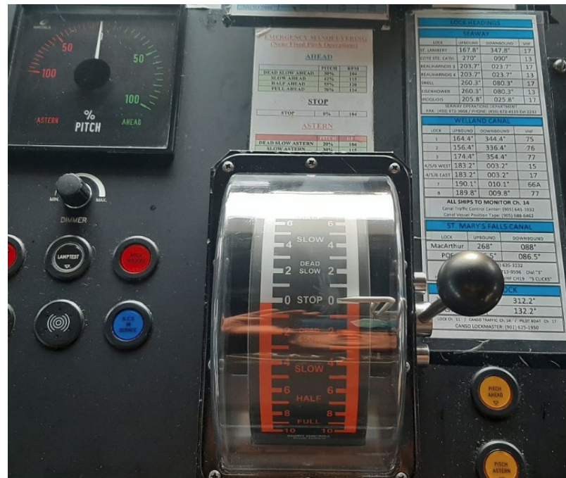
Bridge controls on the Atlantic Huron , including pitch indicator and throttle (rudder control not pictured). (Source: CSL)
