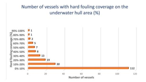
On 44% of vessels surveyed, over 10% of the underwater hull surface was significantly covered with hard fouling. On many vessels, fouling levels were even worse; approximately 15% of vessels had between 10-20% of hard fouling coverage on the hull, 10% of vessels had 20-30% of hard fouling coverage and the remaining 10% of vessels had be-
