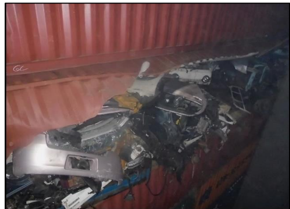
Figure 2: The exploded container in the cargo hold
