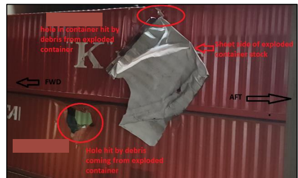
Figure 7: Damages sustained to containers in positions 500516 and 500514
