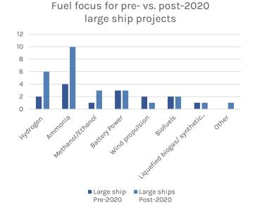
The most significant trend we are seeing with newer large ship technology projects is the post-2020 increase in the uptake of large ammonia vessels. Since the first mapping was released 6 months ago, we have received 4 additional large ammonia ship demonstration projects and are now seeing some of the first orders for these vessels being placed.
