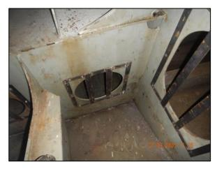
Figure 18: Lightening holes within the starboard bilge space blocked
