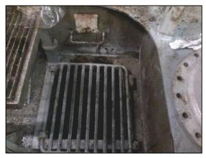
Figure 6b: Access manhole for starboard side bilge alarm sensor
