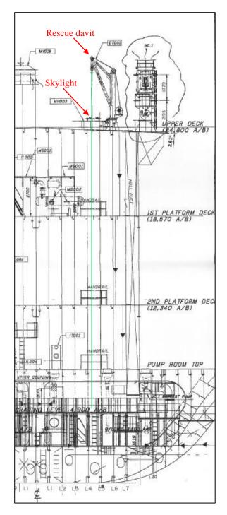
Figure 8: Rescue davit (green line indicates direction through which its wire passes)
