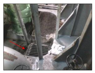
Figure 6a: Access manhole for starboard side bilge alarm sensor (red arrow)
