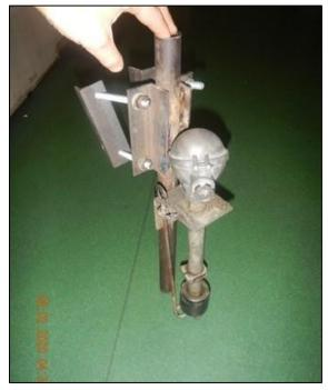
Figure 3: Bilge alarm sensor (representative photograph)
