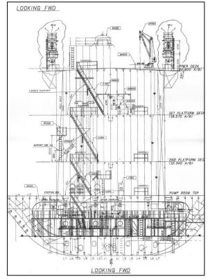
Figure 2: Pump Room Arrangement Plan
