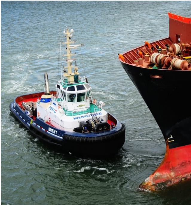
Figure 18: Making tug fast
