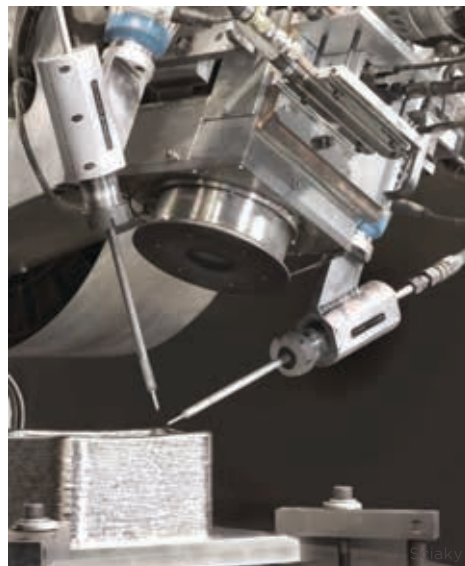
Figure 7 - Electron beam DED system with near-net shape part
