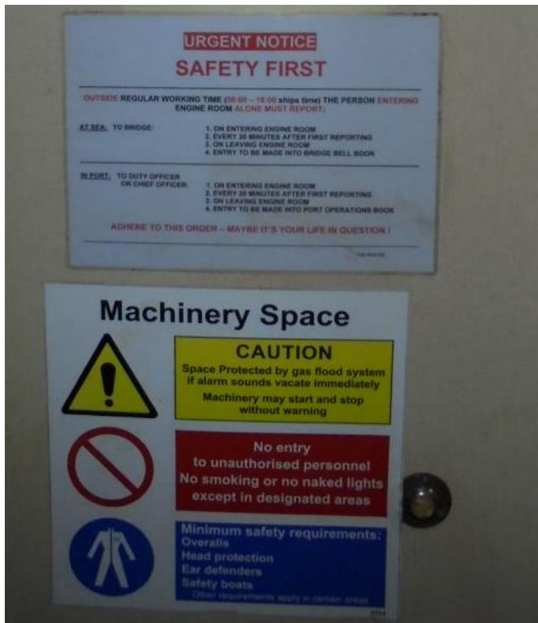
Figure 1 - Entrance door to engine room with instructions
