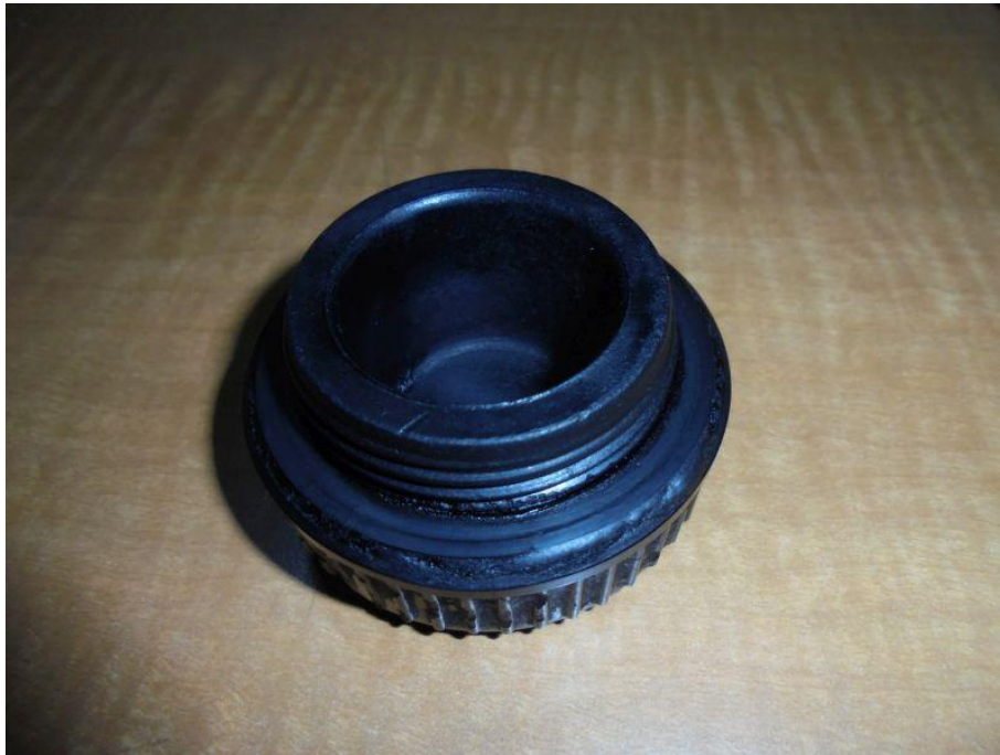
Figure 3 - Plastic plug covering the inspection hole of the sludge discharge line
