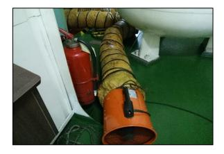
Figure 5: Portable blower used for ventilation
