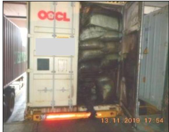
**Figure 5: Right rear door open, showing burnt bags**
