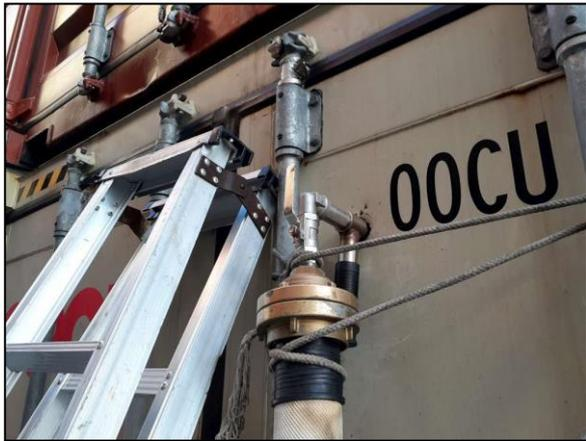
**Figure 3: Water mist lance inserted in container and secured with rope**
