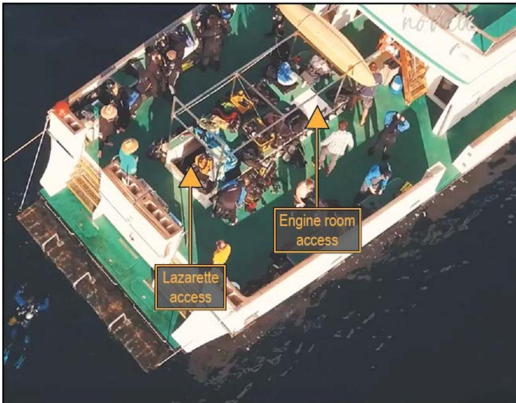
**Figure 4.** Aft main deck of the *Conception* during a previous voyage. (Source: Profundo no Mundo, YouTube, annotated by NTSB)
