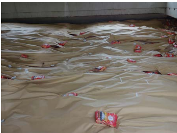
Figure 26: Uppermost layer of bagged cargo topped with kraft paper (photo courtesy of OLDENDORFF CARRIERS GmbH & Co. KG.)
