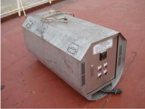
Figure 11: Portable Dehumidifiers (photo courtesy of Neda Maritime Agency Co. Ltd).
