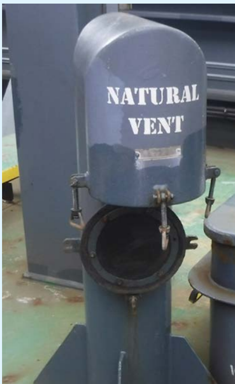
Figure 5: Gooseneck ventilator at cargo hold entrance (photo courtesy of OLDENDORFF CARRIERS GmbH & Co. KG.)
