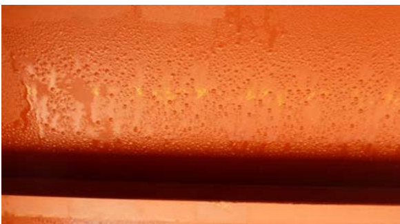
Figure 15: Ship sweat on the underside of the cargo hold hatch cover (photo courtesy of CWA International Ltd)
