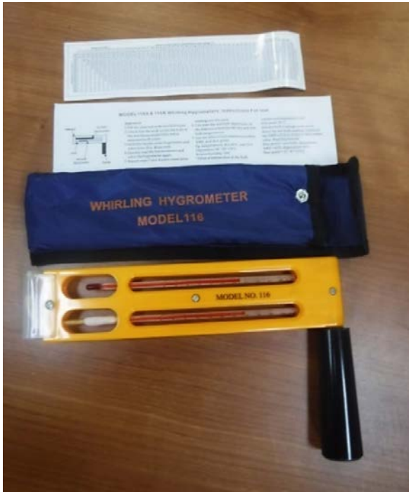
Figure 19: Whirling psychrometer with case, instructions and dew table (photo courtesy of OLDENDORFF CARRIERS GmbH & Co. KG.)
