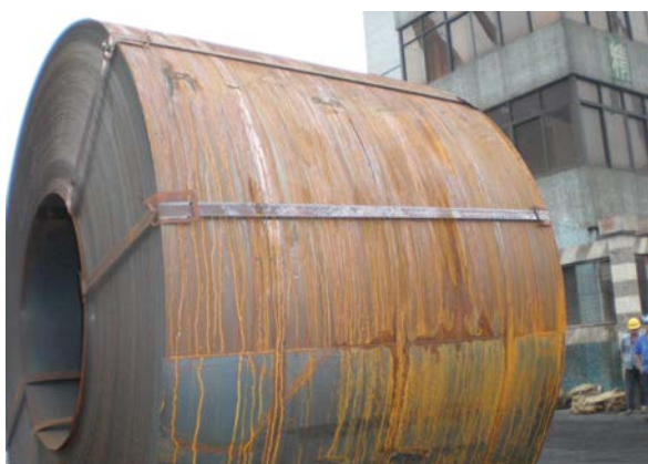
Figure 33: Rust visible on outer surfaces and banding (photo courtesy of The Standard Club)
