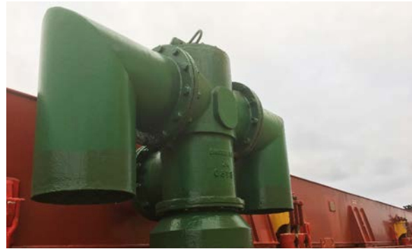
Figure 4: Gooseneck ventilation pipe fitted to hatch cover (photo courtesy of Navios ShipManagement Inc)
