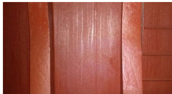
Figure 16: Ship sweat on the shell and side frames of the cargo hold (photo courtesy of Fleet Management Limited)
