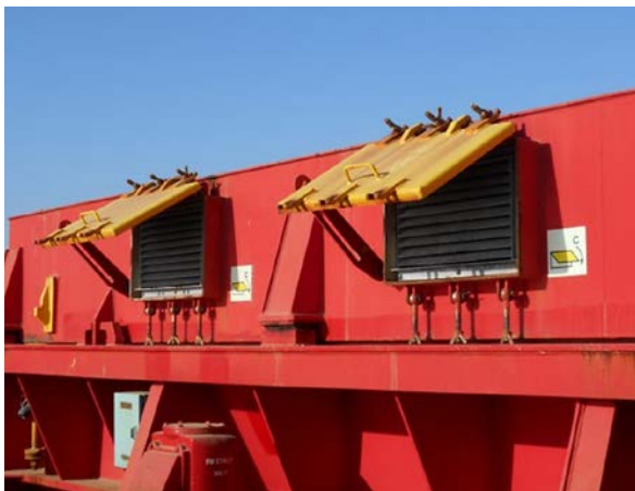
Figure 1: External view of hinged-door ventilator on cargo hold hatch cover side (photo courtesy of Optimum Marine Management Ltd.)
