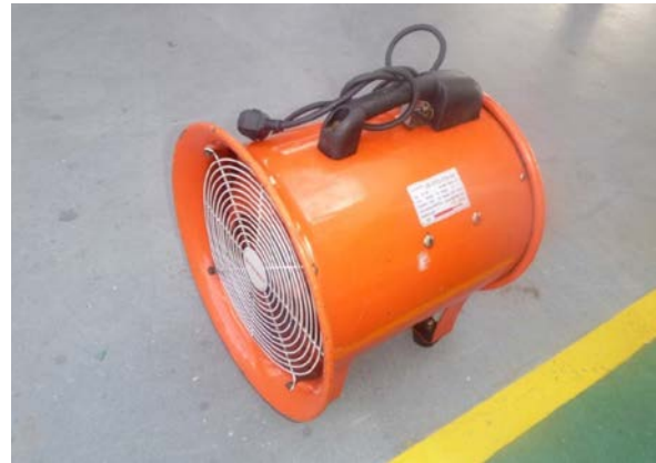
Figure 29: Portable blower for mechanical ventilation (photo courtesy of NYK Line)
