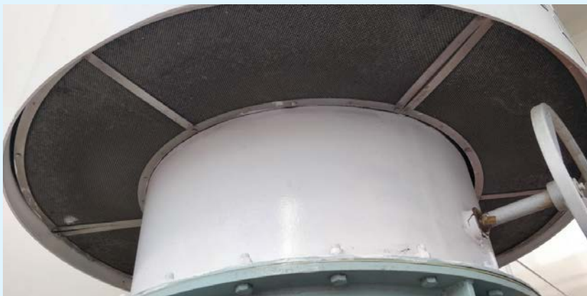
Figure 25: Fixed mechanical ventilator with wire mesh (photo courtesy of Fleet Management Ltd)
