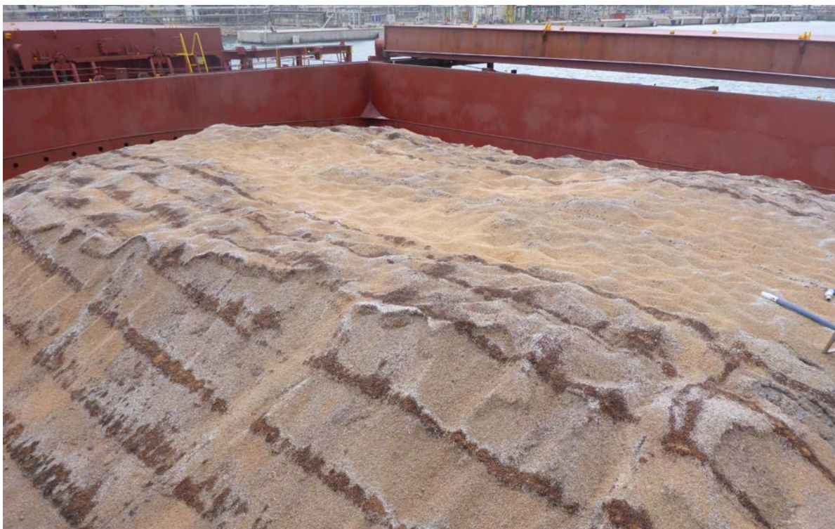
Figure 22: Drip lines from ship sweat on cargo surface (photo courtesy of CWA International Ltd)
