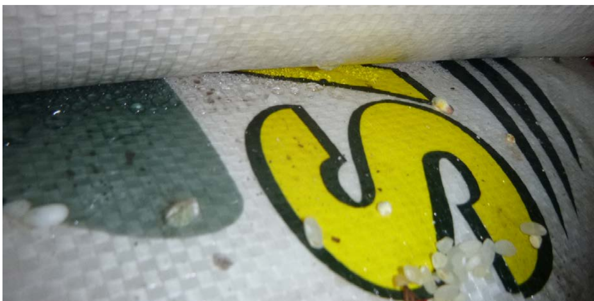
Figure 34: Cargo sweat on rice bags (photo courtesy of CWA International).
