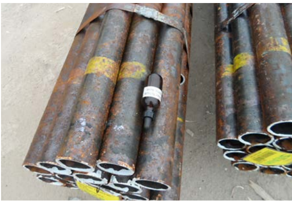
Figure 13: Surface corrosion or rust due to cargo sweat (photo courtesy of The Standard Club)
