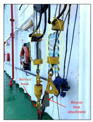
Figure 4: Limit switches for hook travel circled in yellow
