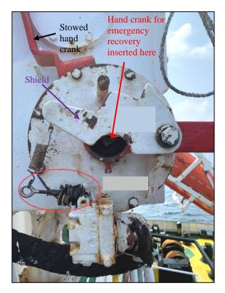
Figure 5: Mechanical safety device – shield for the squared spindle. Once the shield is lifted, the spring deactivates the electrical circuit and the R/B winch is isolated
