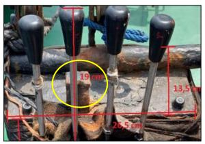
Figure 8: Built-in physical barrier circled in yellow
