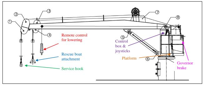
Figure 2: General arrangement of the crane Adapted from: Crane's Instruction Manual
