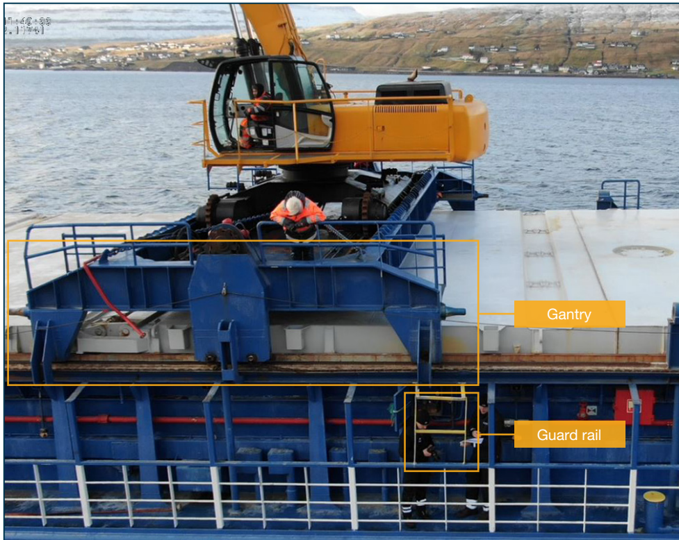
Figure 2: Guard rail and gantry that AB was caught between. Source: DMAIB
