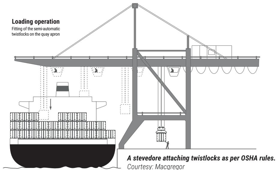
SATs lock automatically and require manually unlocking before unloading begins. FATs do not need any manual operation. All twistlocks have the same safe working load (SWL) of 25 tonnes but the more important figure is the pull-out force or holding power. This is tested by the classification societies. Heavy duty FATs can take higher loads, the safety factor between safe working load and minimum breaking load is four times instead of two times for a light FAT.
