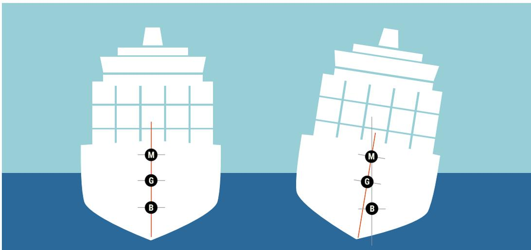
**Ship stability diagram showing centre of gravity (G), centre of buoyancy (B), and metacentre (M) with ship upright and heeled over to one side. As long as the load of a ship remains stable, G is fixed. For small angles M can also be considered to be fixed, while B moves as the ship heels.**
