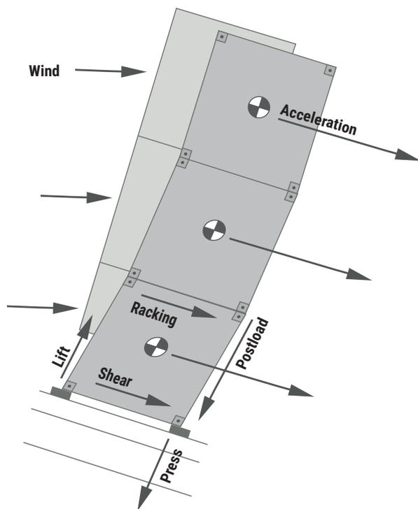
**The mass of the containers will be accelerated by the movements of the ship as a response to the sea conditions.**
