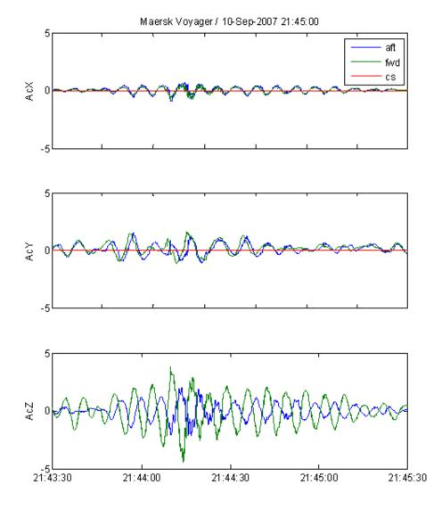
Figure 23 Measured accelerations Maersk Voyager [m/s^2]
