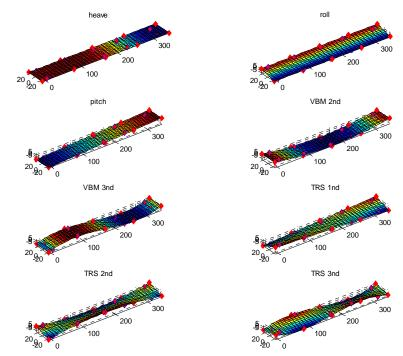
Figure 10 Hull deformation parameterisations
