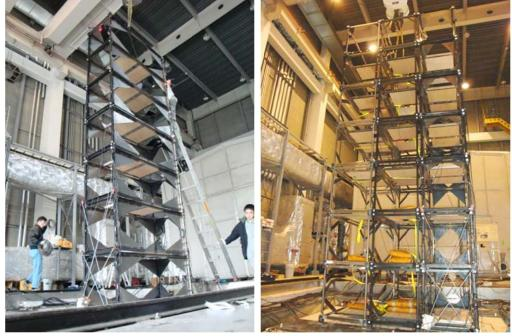
Figure 8 MCS Model scale tests 2-7 tiers, 1-3 rows
