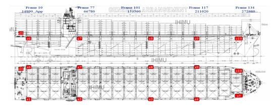
Figure 6 NYK Argus - Accelerometer sensor grid
