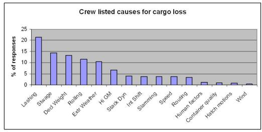
Figure 18 Crew listed causes for cargo losses
