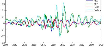
Figure 22 Measured g-loads in transit Schieborg
