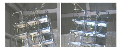
• Peak loads are introduced by impacts when the gaps close due to motions in opposite direction. The more rigid of light stack is found to exhibit peak loads that are factors 2 - 3 higher than the expected values.
