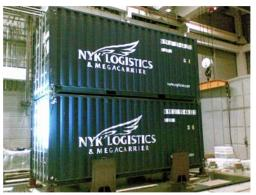
Figure 7 MCS - Full scale container tests 2 tiers
