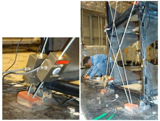
Figure 9 MCS - lashing instrumentation
