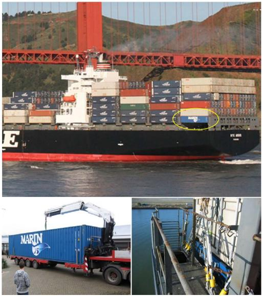
Figure 5 NYK Argus, MARIN instrumented container & lashing rods
