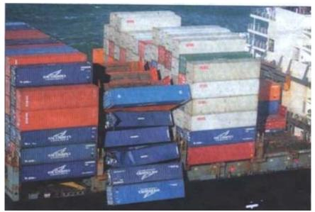
Figure 16 Incidents - Unexplained bay collapse / empty containers
