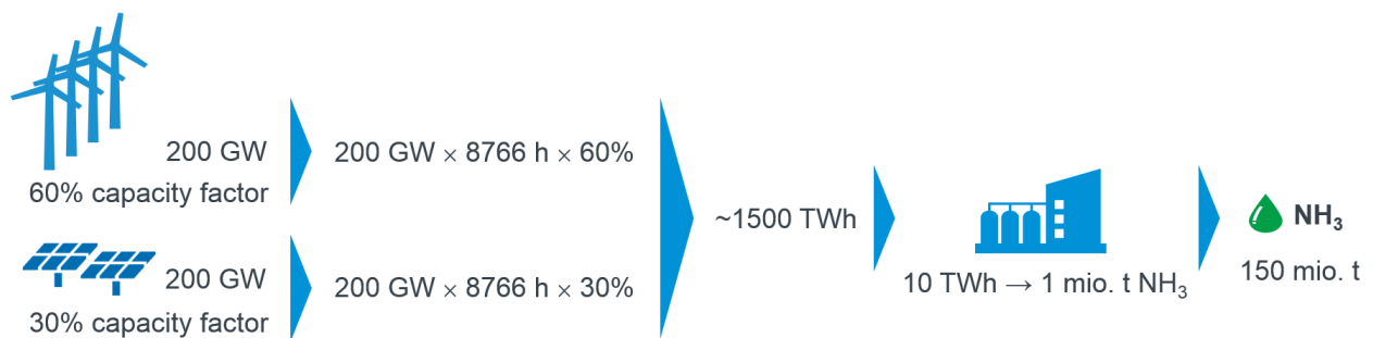
Figure 2. 200 GW of wind and 200 GW of photovoltaics in good sites would be enough to supply 30% of marine fuel consumption.
