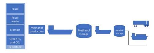
Figure 1: Supply chain of methanol as a maritime fuel.
