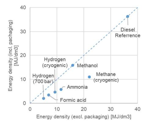
Figure 6: Energy density of different fuel types (TNO (2019)
