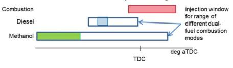
Figure 5: Three combustion technologies for use of methanol in engines. The x-axis is the time represented by the engine crank angle relative to the piston Top Dead Center (TDC). The coloured blocks mark the fuel injections and the combustion process in time.
