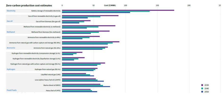
Figure 8: Cost estimation for different production pathways for zero-emission fuels (Lloyd's Register and UMAS (2019a))
