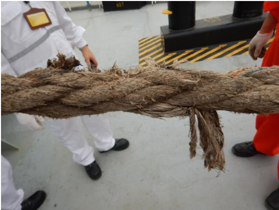
← Partly broken mooring rope
