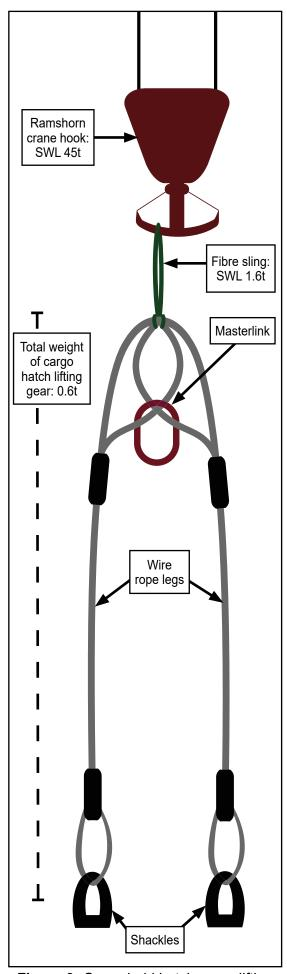
**Figure 3:** Cargo hold hatch cover lifting gear - attachment to crane hook with fibre sling
