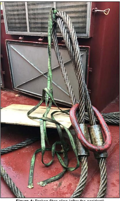
Figure 4: Broken fibre sling (after the accident)
