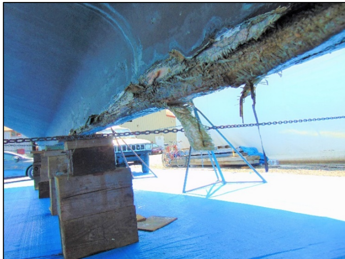
Damage to the keel of the Silver Lining postaccident.
