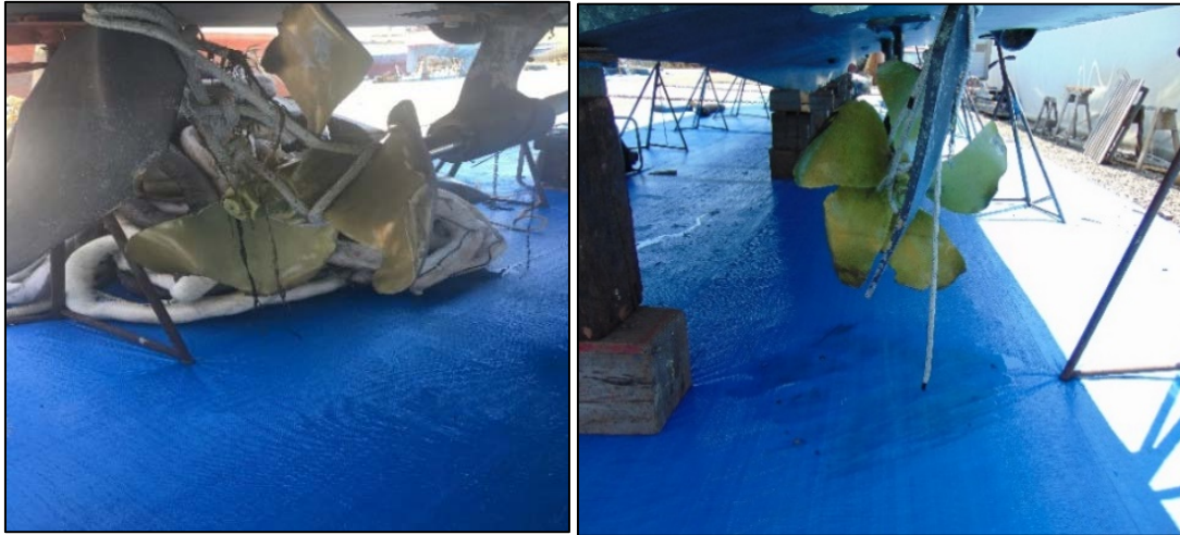
Damage sustained to the port propeller and rudder (left) and starboard propeller and rudder (right) of the Silver Lining following the accident.
