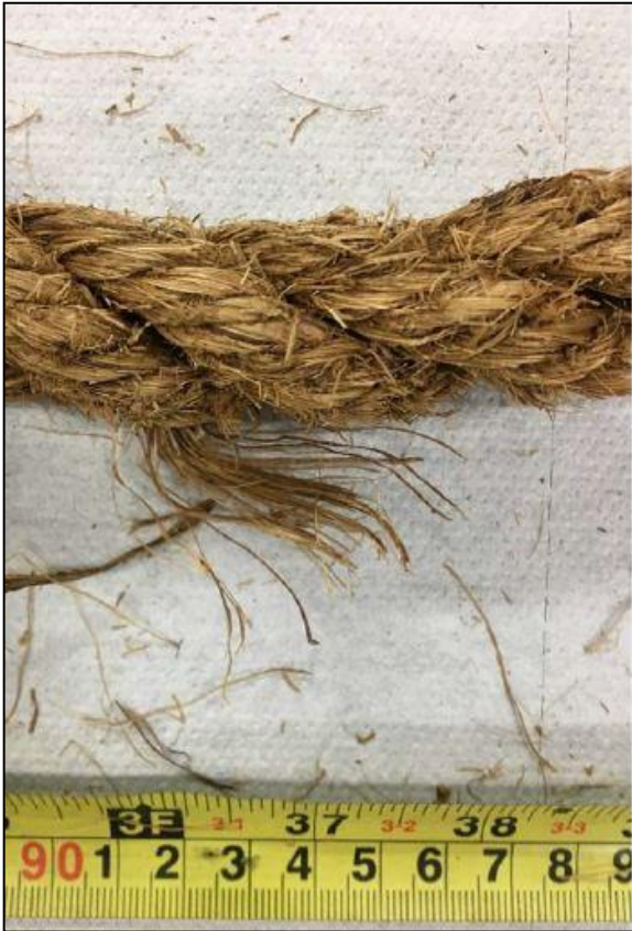
Figure 19: Failed and worn down fibres and strands
