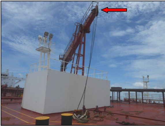
Figure 11: The hose handling crane
