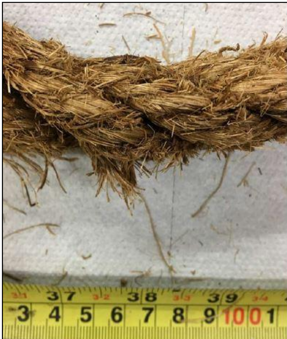
Figure 20: Failed and worn down fibres and strands
