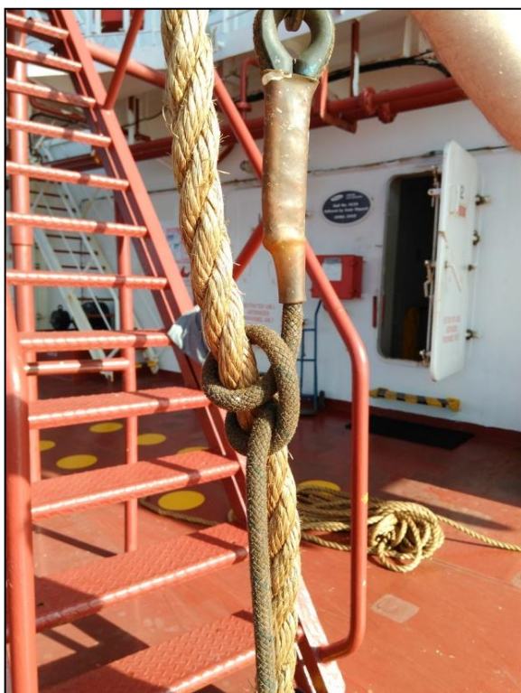
Figure 13: Simulation of safety harness secured to rope B during lowering.
