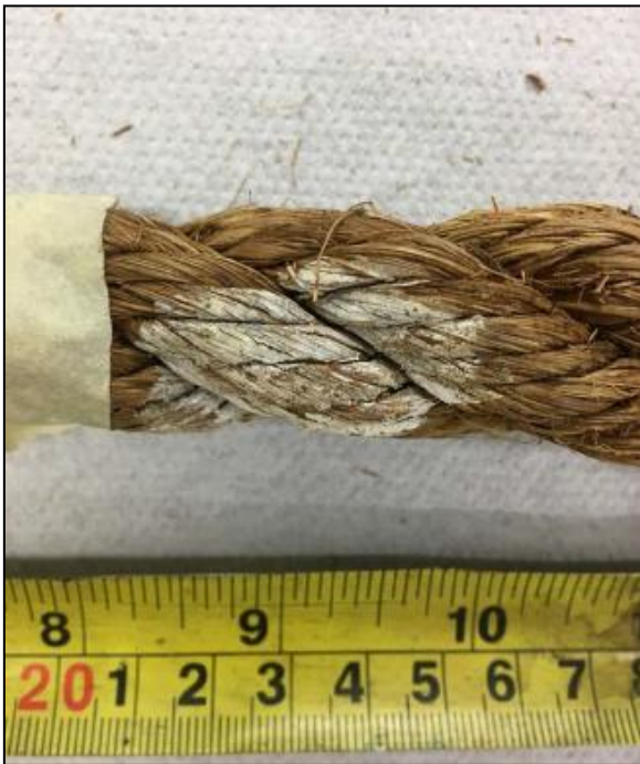
Figure 22: Paint residue on rope sample
