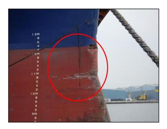
Figure 9: Shell plate damage on Posidana's stem
