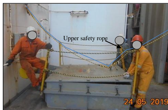
Figure 7: Simulated opening – crew lifting the hatchway cover; with their hands passing in between the stanchions and rope (the line traced in blue was used as a safety measure during the crew's simulation of the accident)
