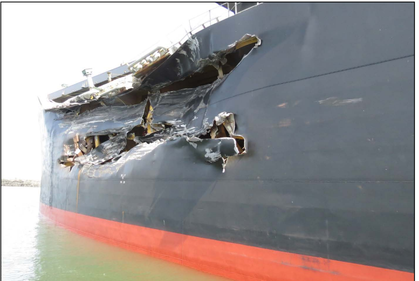
Figure 6: Damage to port side of Cape Mathilde
