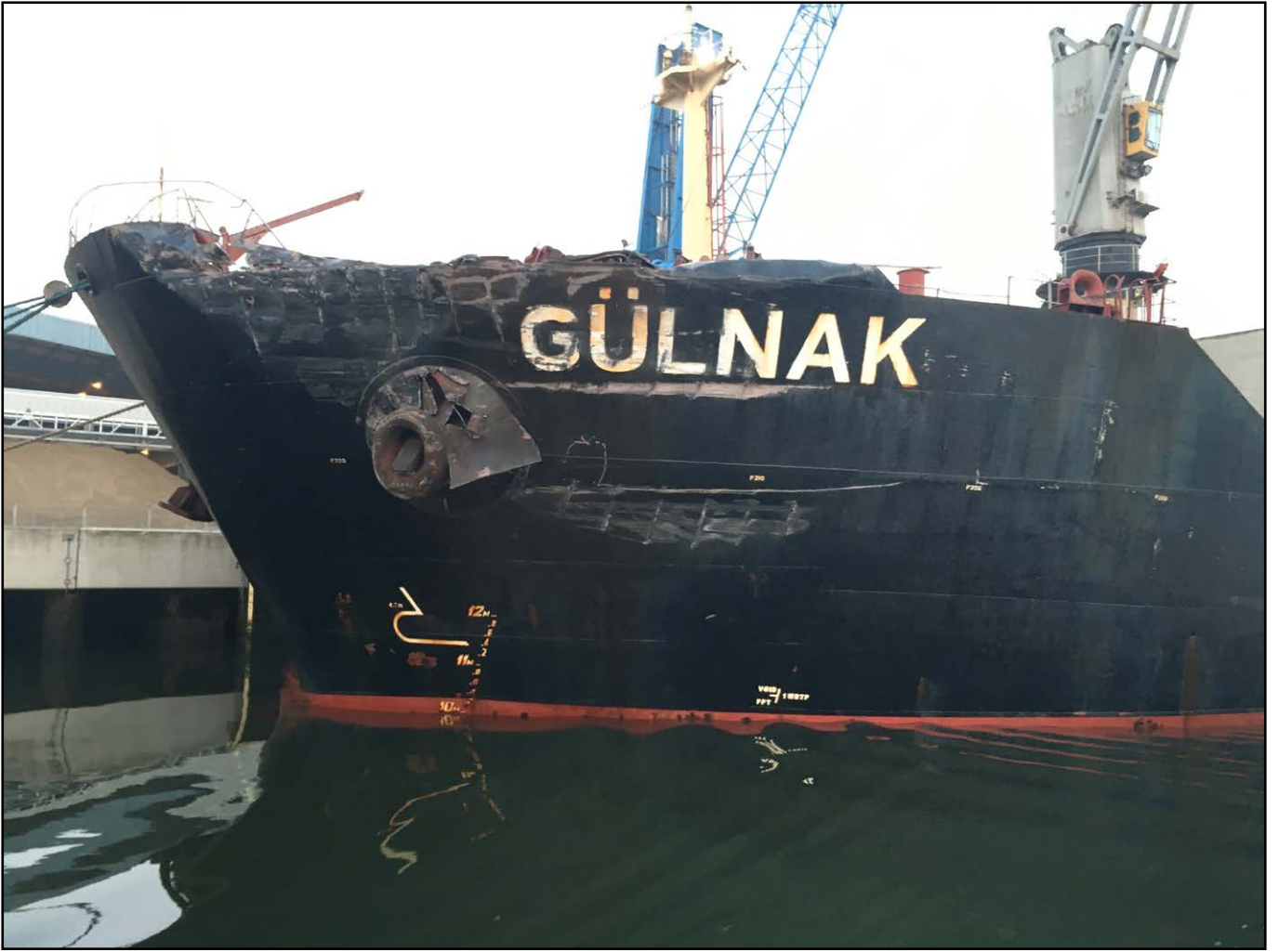
Figure 5: Damage to port bow of Gülnek
