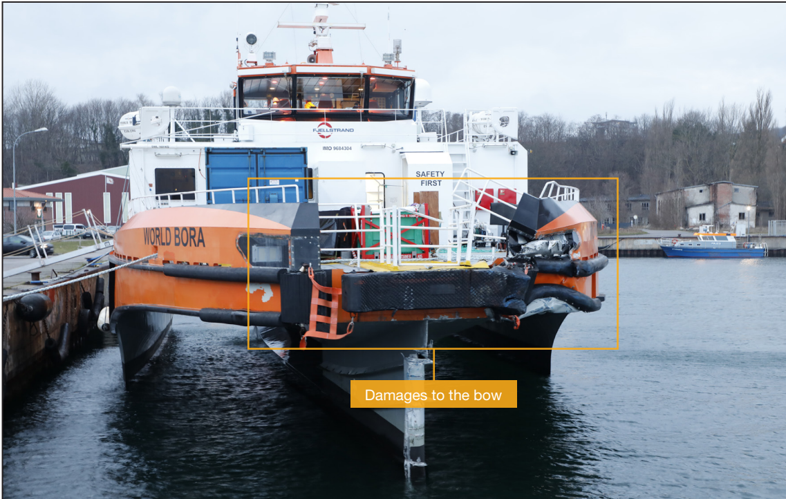
Figure 15: Damages to the bow Source: DMAIB
