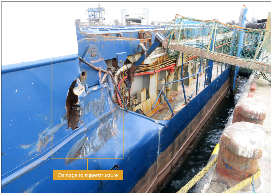
Figure 17: Damages on RABA
