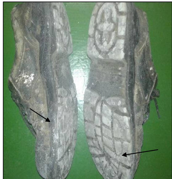
Figure 6: Safety shoes worn by the fatally injured AB. Arrows showing signs of thinning soles
