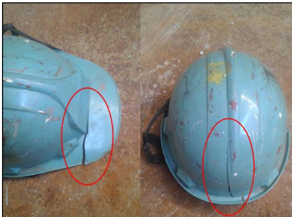
Figure 4: Safety helmet worn by the AB, showing visible cracks front and back
