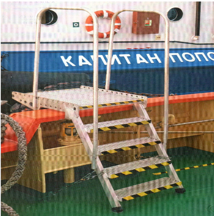
Figure 3: Pilot embarkation platform on KAPITAN AVDYUKOV.
