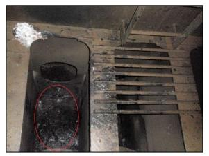
Figure 6: Bilges inside the forepeak tank
