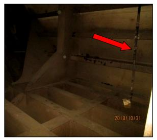
Figure 4: Valve spindle inside the forepeak tank
