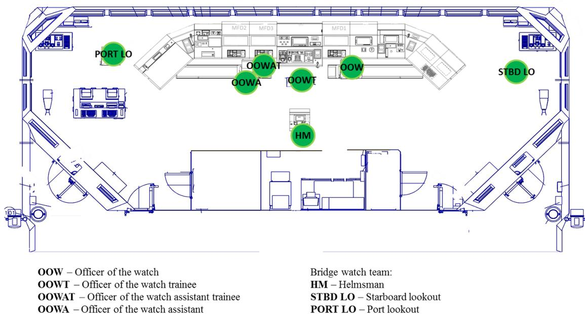
Figure 3: Positions on the bridge of HNoMS Helge Ingstad. Illustration: The Royal Norwegian Navy/AIBN
