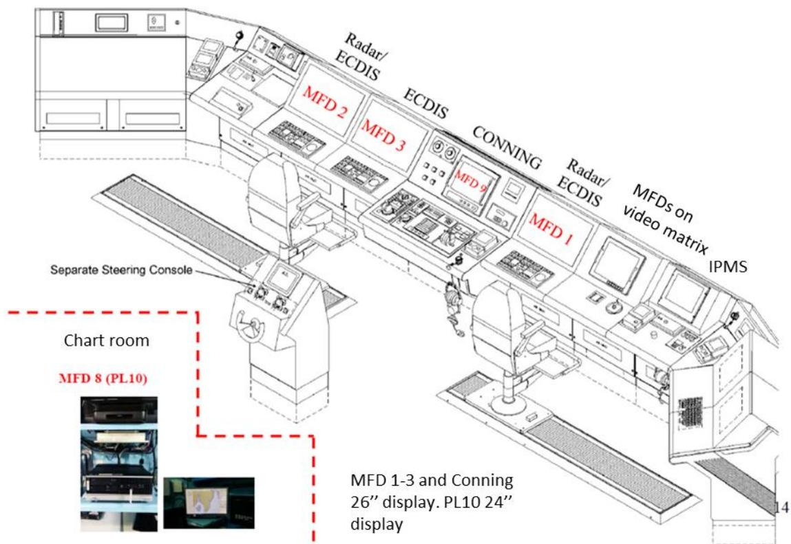
Figure 28: K-Bridge Integrated Bridge System. Illustration: The Royal Norwegian Navy/AIBN
