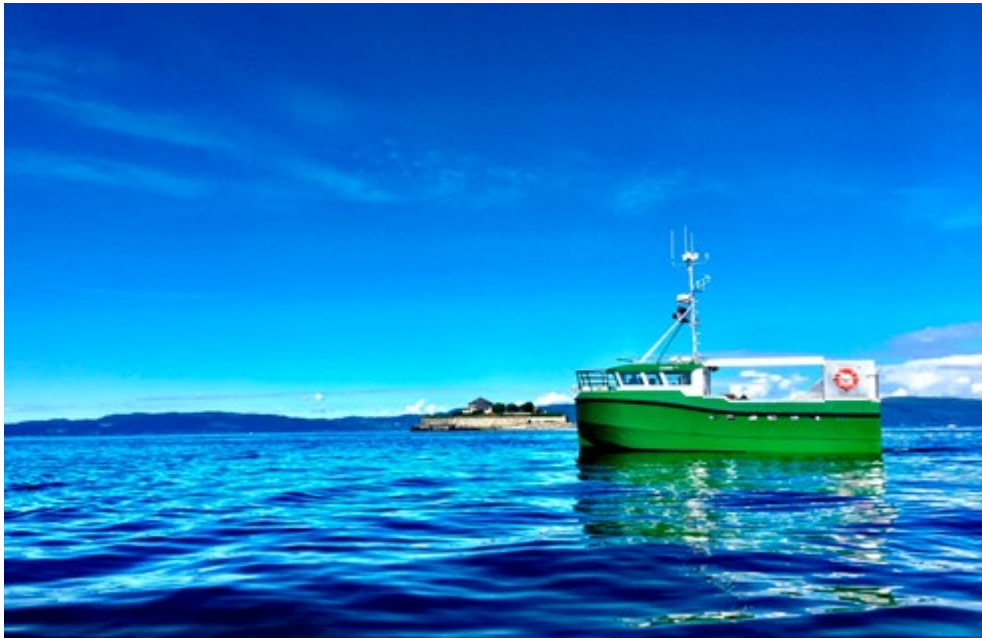
Karoline is the world's first hybrid fishing boat with an electric propulsion system. The vessel is 11 metres long, and has a diesel engine for use to and from the fishing grounds. The battery packs provide the vessel with enough power for two hours fishing and 45 minutes of propulsion. Photo: SIEMENS
