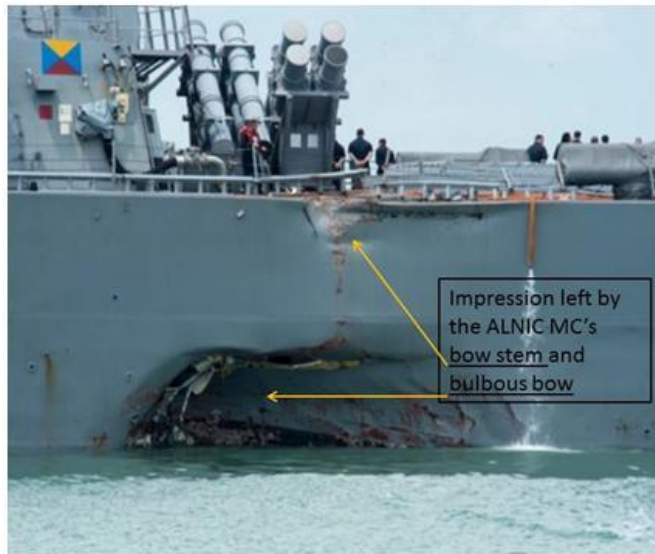
Figure 9 – Point of impact on JOHN S MCCAIN from ALNIC MC
