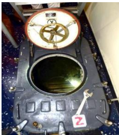
Figure 17—Scuttle and hatch into Berthing 4 showing the space completely flooded
